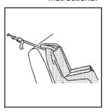
If the position you are using does not have a head restraint and you are using a single tether, route the tether over the seatback.
